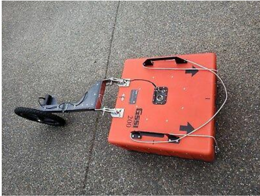
Figure 6 Ground Penetrating Radar shielded Antenna
