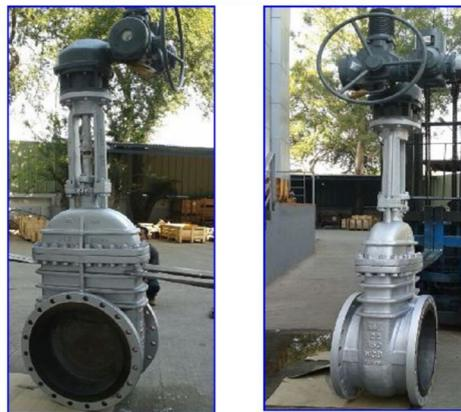
Gate & Globe valve needs special valve with Top flange – To be produced separately
