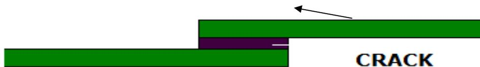
**Figure 3. Geometry of introduced crack in adhesive layer**
